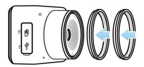
**1** Securely attach an add-on filter by rotating it clockwise onto the UV filter or the focus ring.
