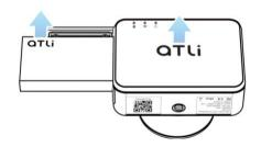
**3** Use the battery to push down the yellow latch until it is fully retracted, allowing space for the battery to be inserted into the battery compartment.
